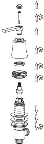
2. From below, insert each of the valve stems into their prepared mounting holes, as shown. Ensure that the hot valve (red) is on the left, and the cold valve (blue) is on the right. From above, thread the upper lock nut, lock sleeve, and hex nut onto the stems.
